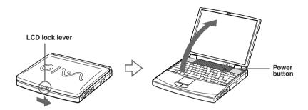
Press the power button on top of the computer until the green power indicator light turns on.
